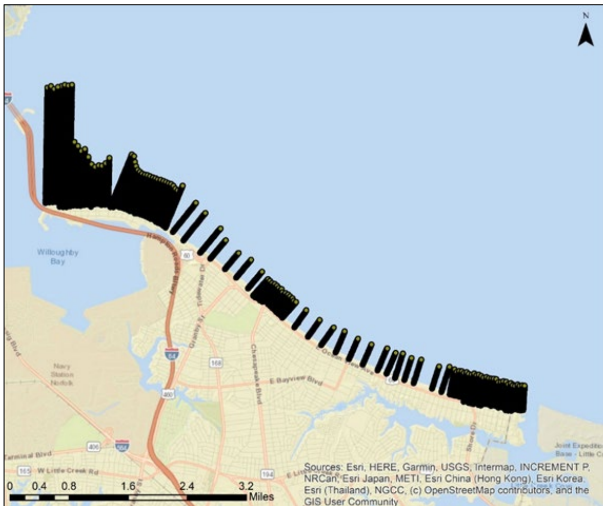
Fig. 9 Plan view of topographic/bathymetric transects survey.
