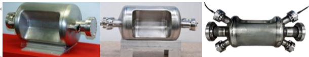
Figure 1: Built and tested RFD proof-of-principle cavities. From left, 400MHz LHC Hi-Lumi crab cavity, 499 MHz JLab deflecting cavity, 750 MHz JLab MEIC crab cavity.
