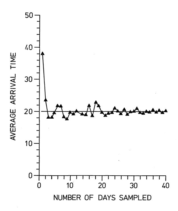
time density  $(\cdot \bar{t}_j)$  may be well above or below the population mean of the distribution resulting in a broader amplitude. As the number of days sampled approaches the population size, m, the wave function dampens and the observed values match the expected population mean (j = m).
