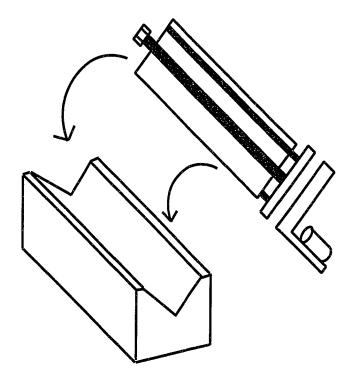
Fig. 3.6 Barrel holder used to orient and cut the Ge single crystals. The barrel holder fits into a V-block that helps keep it stationary during cutting and orientation.
