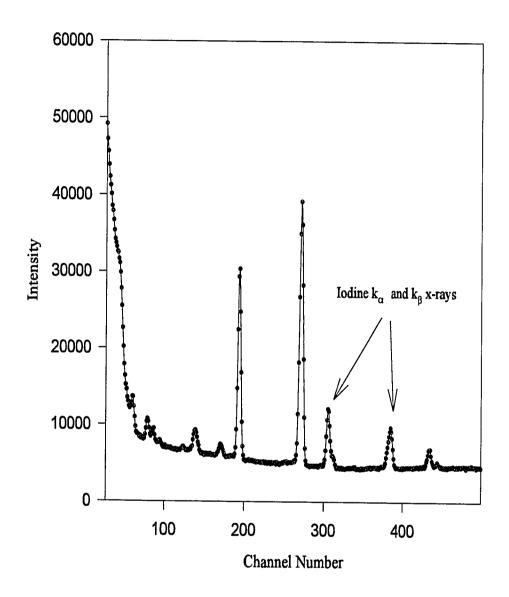
Fig. 5.17 Pulse-height spectrum showing the iodine x-rays that come from ionization of the NaI detector.
