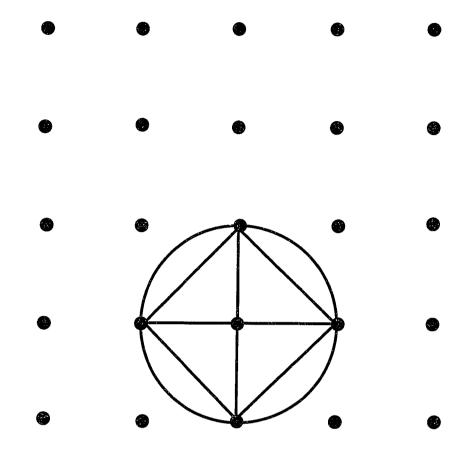
Fig. 2.3 Ewald's Sphere of Reflection showing simultaneous diffraction. Since the sphere intersects with four reciprocal lattice points, there will be a four beam diffraction.
