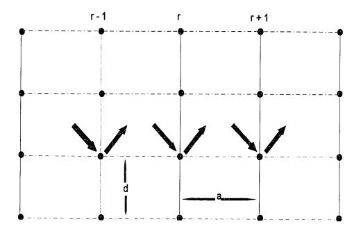
Fig. A.3 Schematic representation of the diffracted and forward diffracted wavefields inside the crystal. This construction is useful for finding recursion relationships for the forward diffracted and diffracted waves.
