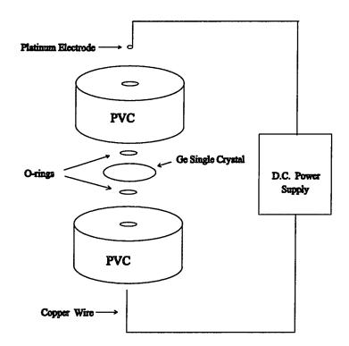
Fig. 3.9 Schematic of the electroplating cell used to apply radioactive <sup>73</sup>As onto the Ge single crystal.
