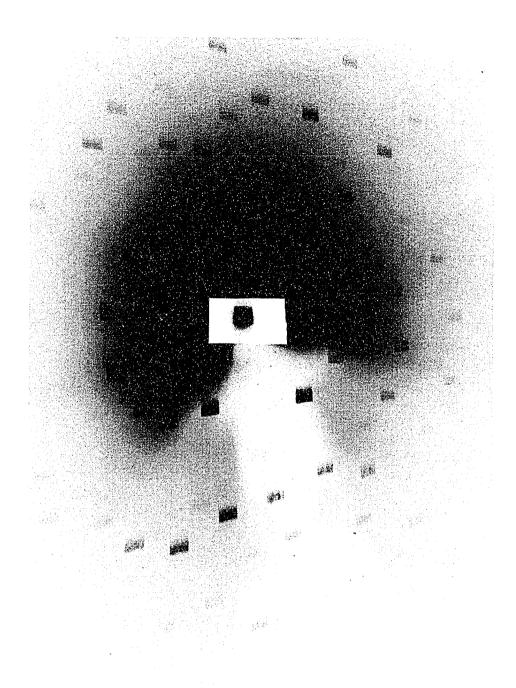
Fig 3.2 Laue transmission photograph. The crystal being used is one of the <sup>57</sup>Co doped Fe single crystals.
