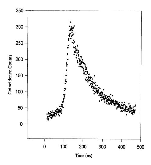
Fig. 5.19 Time-filtering curve using the 6.4 keV x-ray of <sup>57</sup>Fe. The prompt has been eliminated by switching the Ge solid state detector and the NaI detector.
