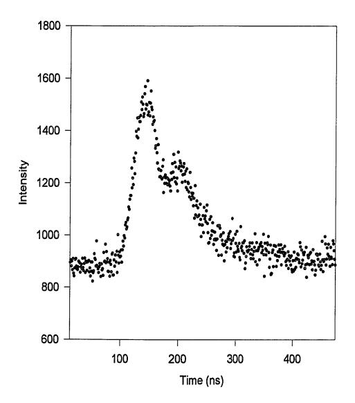
Fig. 5.18 Time-filtering curve collected with the low energy windows set on the Compton background.
