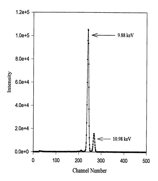
Fig. 5.3 Pulse-height spectrum of  $^{73}\text{Ge}$  showing the  $K_{\alpha}$  and  $K_{\beta}$  x-ray peaks.
