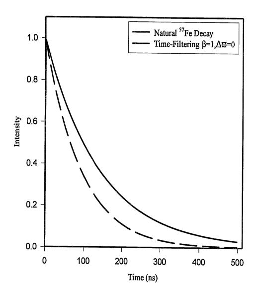
Fig. 4.1 Time-filtering curve for  $\beta=1$  and  $\Delta\omega=0$ . The solid line is the natural <sup>57</sup>Fe decay.
