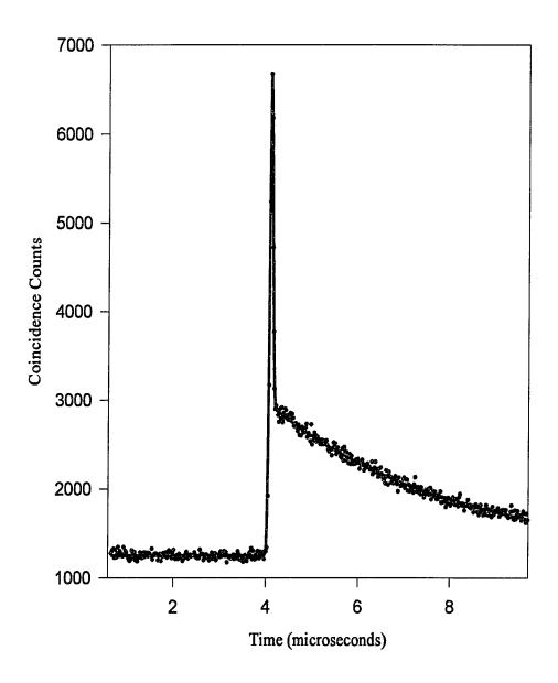
Fig. 5.9 Time-filtering curve using the 9.88 keV <sup>73</sup>Ge x-ray.
