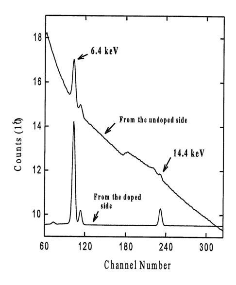
Fig. 3.1 Pulse-height spectrum showing the transmitted <sup>57</sup>Fe radiation. A pulse-height spectrum from a standard <sup>57</sup>Co source is superimposed on the graph to help show the locations of the peaks.
