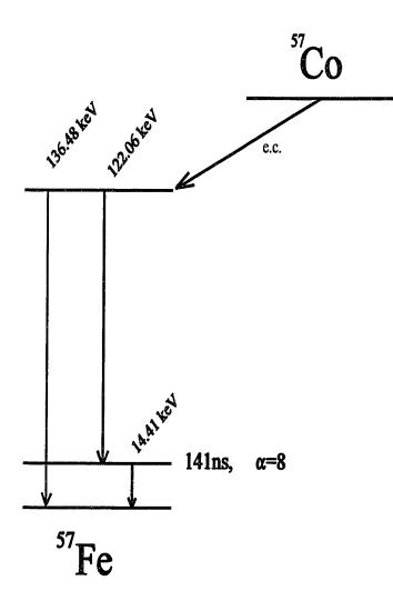
Fig. 5.1 Schematic diagram of the <sup>57</sup>Co-<sup>57</sup>Fe decay.
