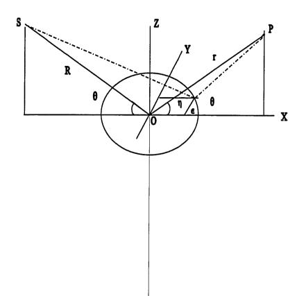
Fig. A.1 The reflection of x rays from a plane can be described in terms of a Fresnel zone. In this figure, the Fresnel zone in a horizontal plane.
