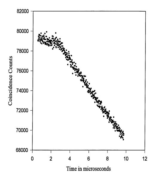
Fig. 5.6 Background shape of coincidence measurements when the stop rate is larger than the inverse of the full scale time range set on the TAC.
