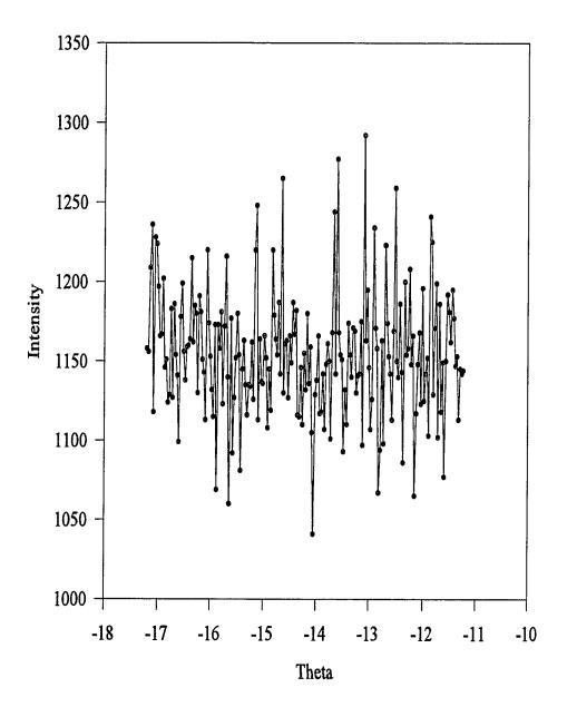
Fig. 3.11 Borrmann scan of the 13.26 keV gamma ray. A peak should occur at 13.52°. No peak is present which may be due to the small signal to noise ratio.
