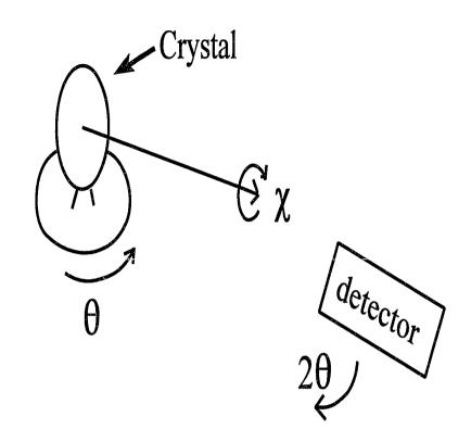
Fig. 3.5 Block diagram defining the angles used on the goniometer. The  $\theta$  axis corresponds to a rotation about the crystal mount. The  $\chi$  axis is a rotation about the axis of the crystal face, and  $2\theta$  is the angle of the detector.
