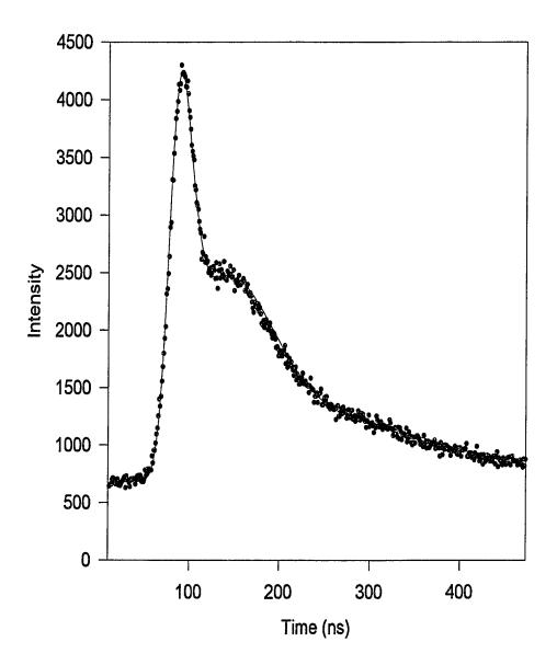
Fig. 5.13 Time-filtering curve for <sup>57</sup>Fe using a Ge solid state detector on one side of the coincidence circuit. Special care was taken to reduce the resolution time of the circuit to compensate for the slowness of the Ge detector.
