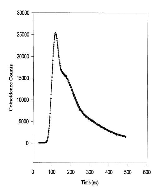
Fig. 5.11 Plot of the <sup>57</sup>Fe gamma-ray time-filtering curve using NaI on both branches of the coincidence circuit.
