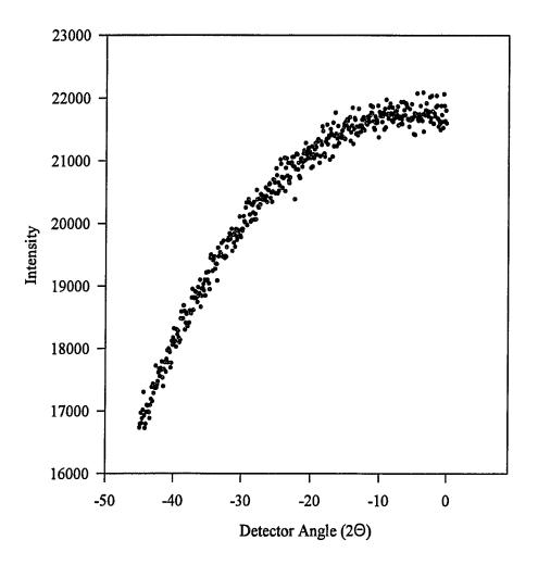
Fig. 3.10 Laue scan of the transmitted 53 keV radiation for a Ge (111) crystal. A Bragg peak is expected at 3.35°. No peak is present, however the shape suggests the radiation had to traverse the crystal since at larger angles the radiation had more material to travel through.
