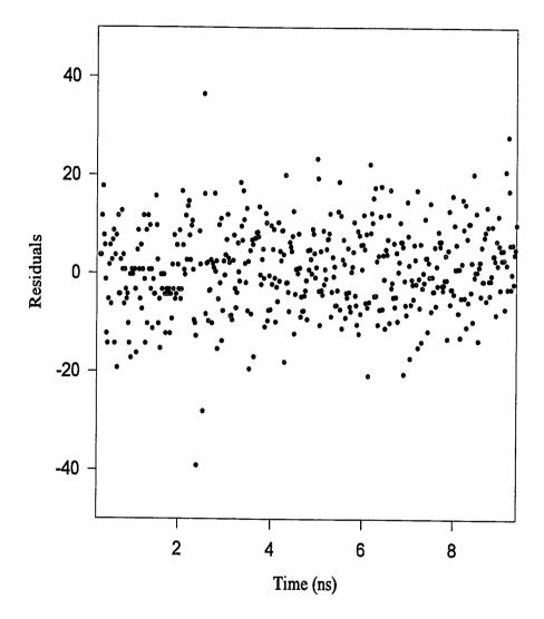
Fig. 5.8 A plot of the residuals from the time-filtering fit for the  $^{73}$ Ge 13.26 keV timing curve.
