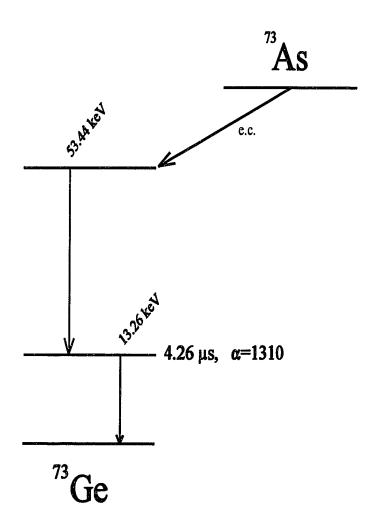
Fig. 5.2 Schematic diagram of the  $^{73}$ As- $^{73}$ Ge decay.
