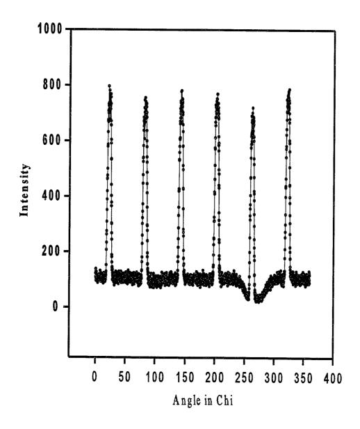
Fig. 3.8 Borrmann scan of the Ge (111) crystal showing the three-fold symmetry axis.
