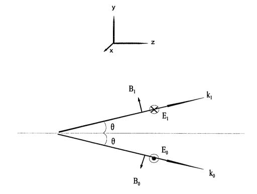
Fig 2.4 Construction of a Bragg reflection showing the orientation of the electric and magnetic fields associated with each wavevector.
