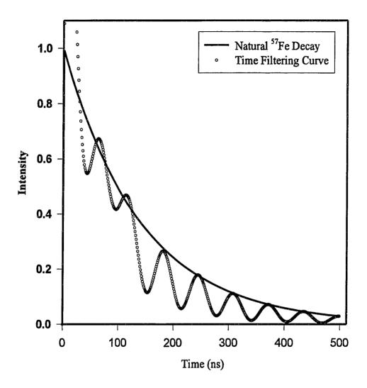
Fig. 4.3 Time-filtering curve for  $\beta$ =10 and  $\Delta\omega$ =7. The solid line is the <sup>57</sup>Fe natural decay. The time-filtering curve oscillates about the exponential curve. Notice that at very early times, more radiation is present when a filter is in place that would be if the filter were not present.
