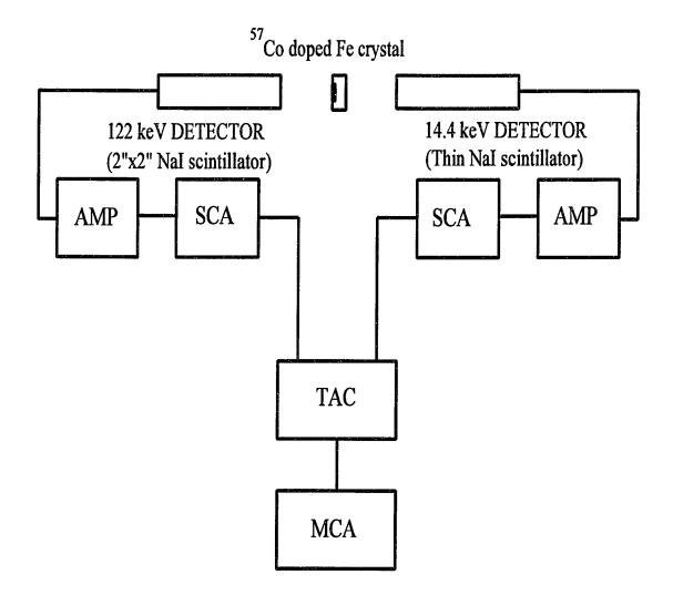
Fig. 5.5 Schematic of the coincidence setup. For some cases, the low energy side of the circuit used a Ge solid state detector instead of a NaI detector.
