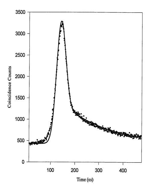
Fig. 5.16 Time-filtering curve for <sup>57</sup>Fe using the 6.4 keV x-ray. The solid line is an attempt at fitting by the Hamermesh theory.
