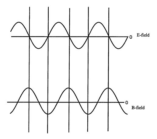
Fig. 2.5 The standing wave in the crystal produces an electric field that is near zero at the atomic sites, and magnetic field that is large at the atomic sites. The vertical lines represent the planes of atoms. If the radiation is resonant with the nuclei, the radiation will couple strongly to the nuclei if the transition is magnetic dipole (M1).
