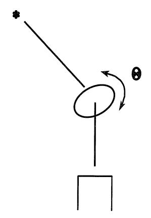
Fig 3.4 Schematic representation of the procedure for measuring a rocking curve. The detector is held fixed while the crystal is rotated about an axis perpendicular to the plane defined by the incident beam and the diffracted beam.
