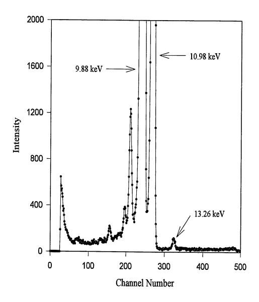
Fig. 5.4 Pulse-height spectrum showing the 13.26 keV <sup>73</sup>Ge gamma ray.
