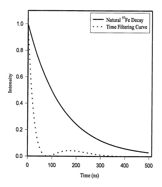
Fig. 4.2 Time-filtering curve for  $\beta$ =10 and  $\Delta\omega$ =0. The solid line is the <sup>57</sup>Fe natural decay.
