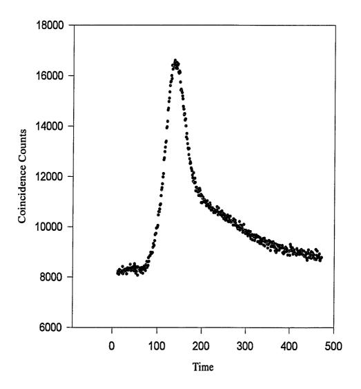
Fig. 5.15 Time-filtering curve using the 6.4 keV of <sup>57</sup>Fe. This spectrum was collected with NaI on both sides of the coincidence system. Some effort must be made to eliminate the prompt that is present in the spectrum.
