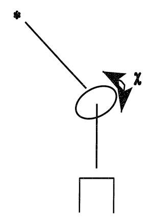
Fig. 3.7 Scan about the  $\chi$  angle to search for Borrmann transmissions. The crystal is oriented in the Laue geometry and rotated about the face axis. As the planes become aligned, the Bragg condition is satisfied, and an intensity peak is recorded in the detector.
