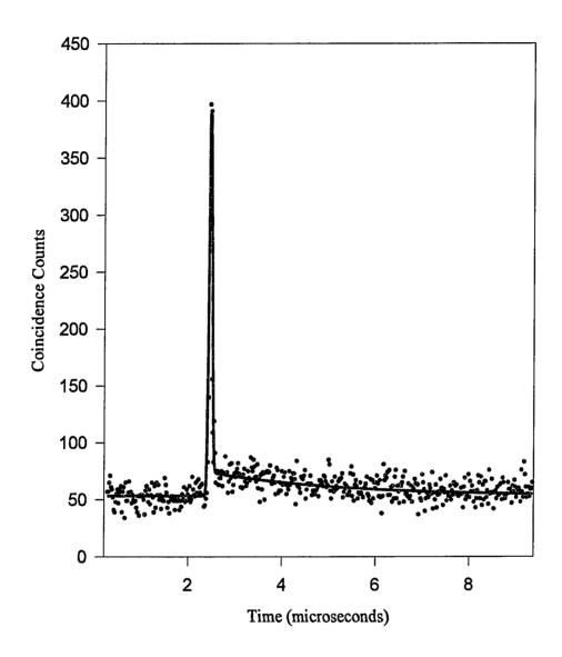
Fig. 5.7 Time-filtering Curve using the 13.26 keV <sup>73</sup>Ge gamma ray. The count rate is exceedingly poor partially due to the high internal conversion coefficient.
