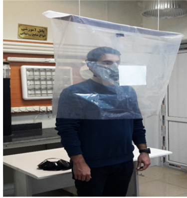
Fig. 1. The participant was inside the test hood during the IAA fit testing procedure.
