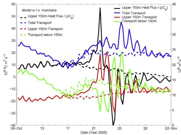
**Figure 3.** Model volume (right-side scale) and heat transports ( $\rho_o C_p$ ) through the Yucatan Channel during Wilma. Solid curves are for model with Wilma; dashed curves are without Wilma. The upper 150 m heat flux is defined as  $\rho_o C_p \int \int v(T - 26) dx dz$ , where  $v$  is the velocity normal to the transect,  $T$  is temperature, and vertical integration is from  $z = -150$  m to the surface.
