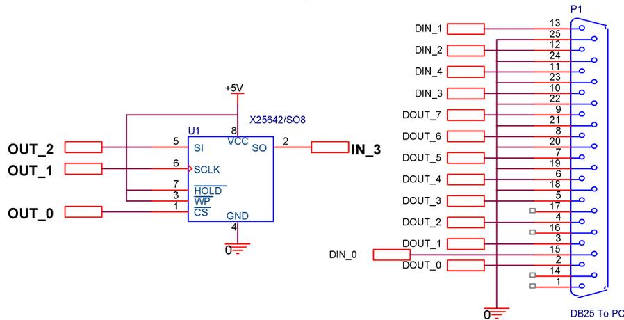
**Figure 4. PC Parallel Port to Serial EEPROM Interface**
