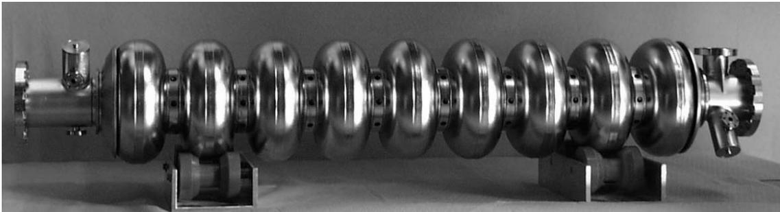
Figure 5: A 1.3 GHz 9-cell SRF cavity developed by the TESLA collaboration in 2000 [24]. This design is still widely used in accelerator facilities around the world.
