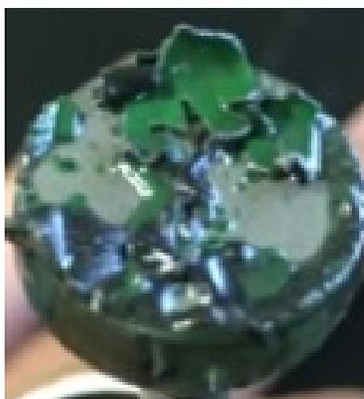
Figure 72: Example of a sample after plasma etching. The color indicates chlorine contaminants on the surface.
