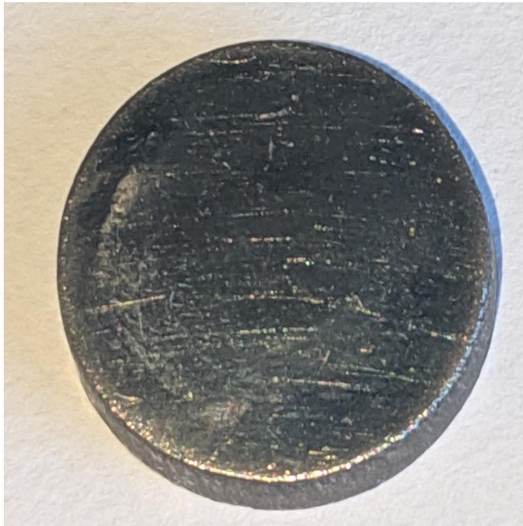
Figure 49: A picture of a Nb coupon sample polished to 1 micron surface roughness. A mirror-like surface can be seen, along with surface defects like pits and trenches.
