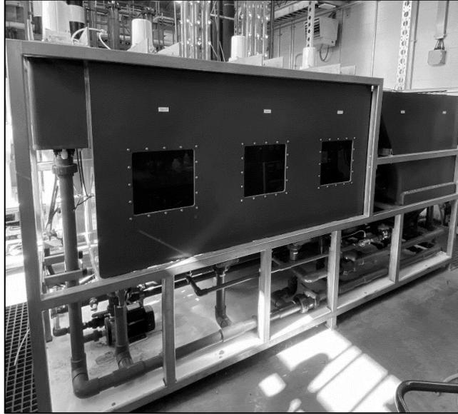
**Figure 12: Intuitech Flocculation Sedimentation Pilot**
