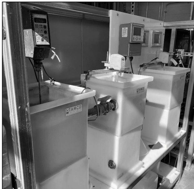
**Figure 13: Rapid Mix and Flocculation Basins for Direct Filtration Pilot**
