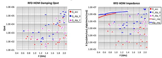
Figure 5: The  $Q_{ext}$  and impedance of the HOMs.
