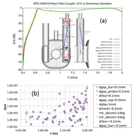
Figure 6. Sensitivity of  $Q_{ext}$  on coupler dimension errors.
