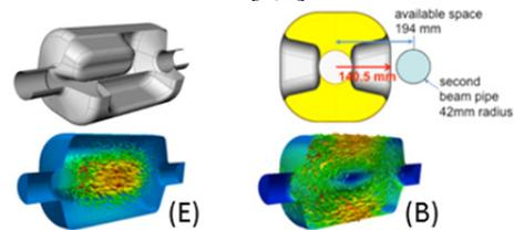
Figure 1: RFD crab cavity and the field patterns.
