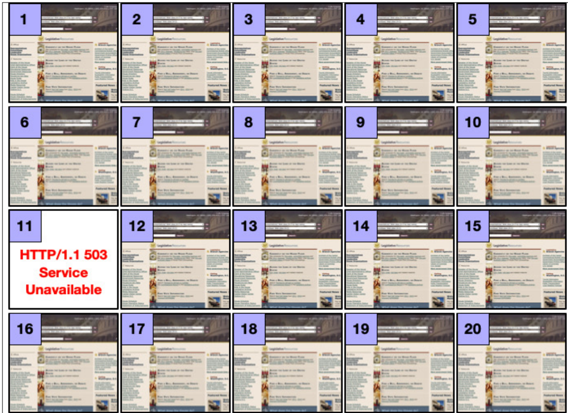
Fig. 67: An example of a transient error. Replaying a memento 20 times. The archive replies with HTTP 503 Service Unavailable at download 11.
