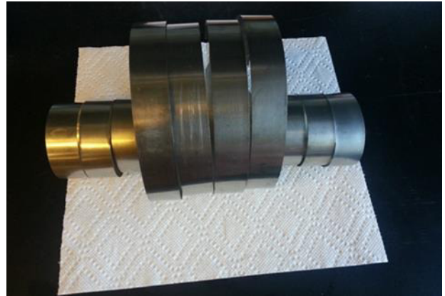
Figure 3: Different diameter Nb samples to be placed in the pill box cavity.
