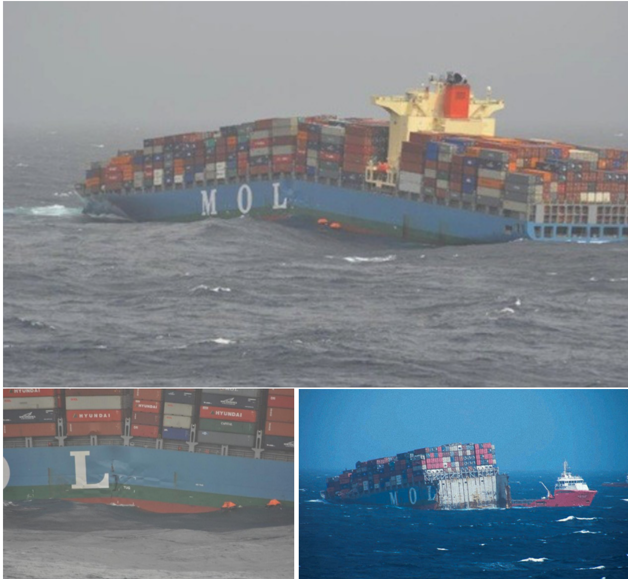
FIG. 14: On June 17, 2013, Mitsui O.S.K. Lines' 2008-built MOL Comfort began suffering from severe hogging and broke in two while underway from Singapore to Jeddah [29].
