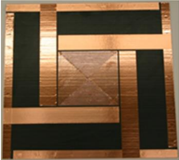
Fig. 1. Actual Test Panel with 7 inch SansEC (shown unpainted)
