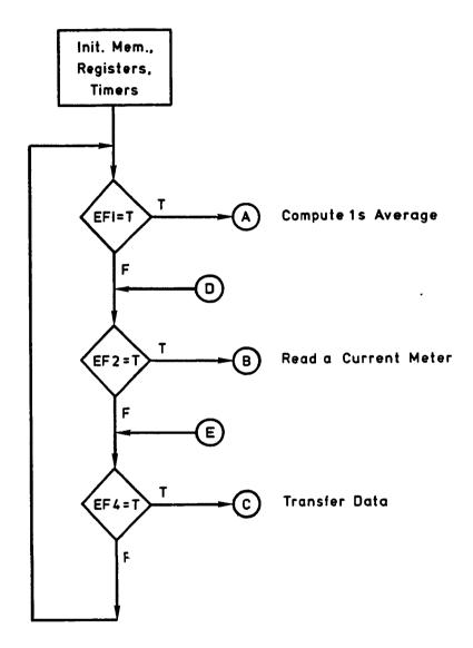
Figure 4b. Flow chart of the data read subroutine.
