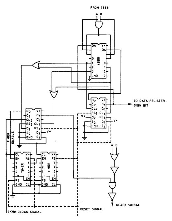
Figure A7. Timer output, data lines, and data bus circuitry.
