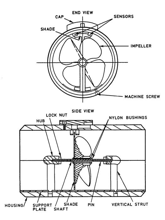
bushings, and a thin stainless steel shade integral to the impeller that interrupts the light beam.
