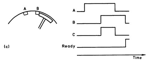
Figure 3. Timing diagram to illustrate the problem when there is no time overlap between channel A and B.
