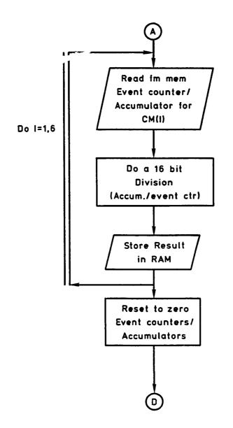
Figure 4d. Flow chart of the data transfer subroutine.
