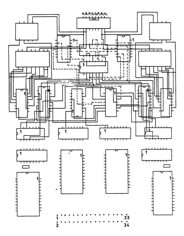
Figure A6. Timer controll logic circuitry.
