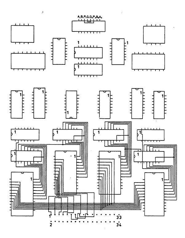
Figure A8. Controll signals to and from the microprocessor board via the interface.
