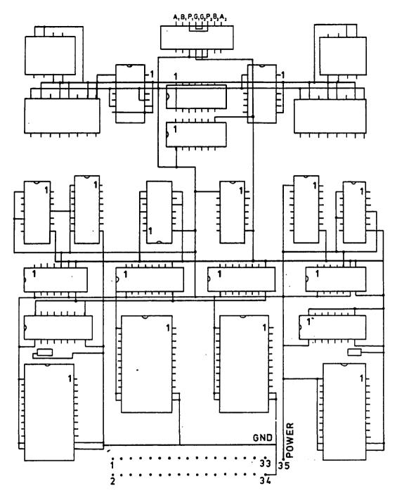
Figure A5. Logic circuits that controll the timing devices and generate the ready signals. (See Figure A6 for details of the logic circuitry).
