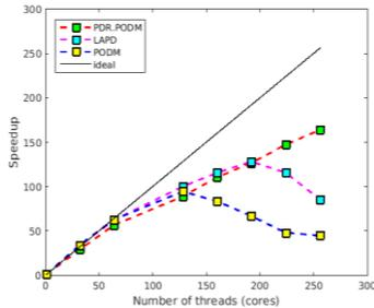
Figure 4: Weak Speedup comparison of PODM optimizations for meshes that vary from 3M tetrahedra to 745M tetrahedra on 256 cores.
