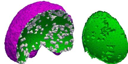
Figure 6 (a) : The curved surface is treated as a constrain. Like PCDM for each encroaching element (white tetrahedron) a split message has to be sent.
