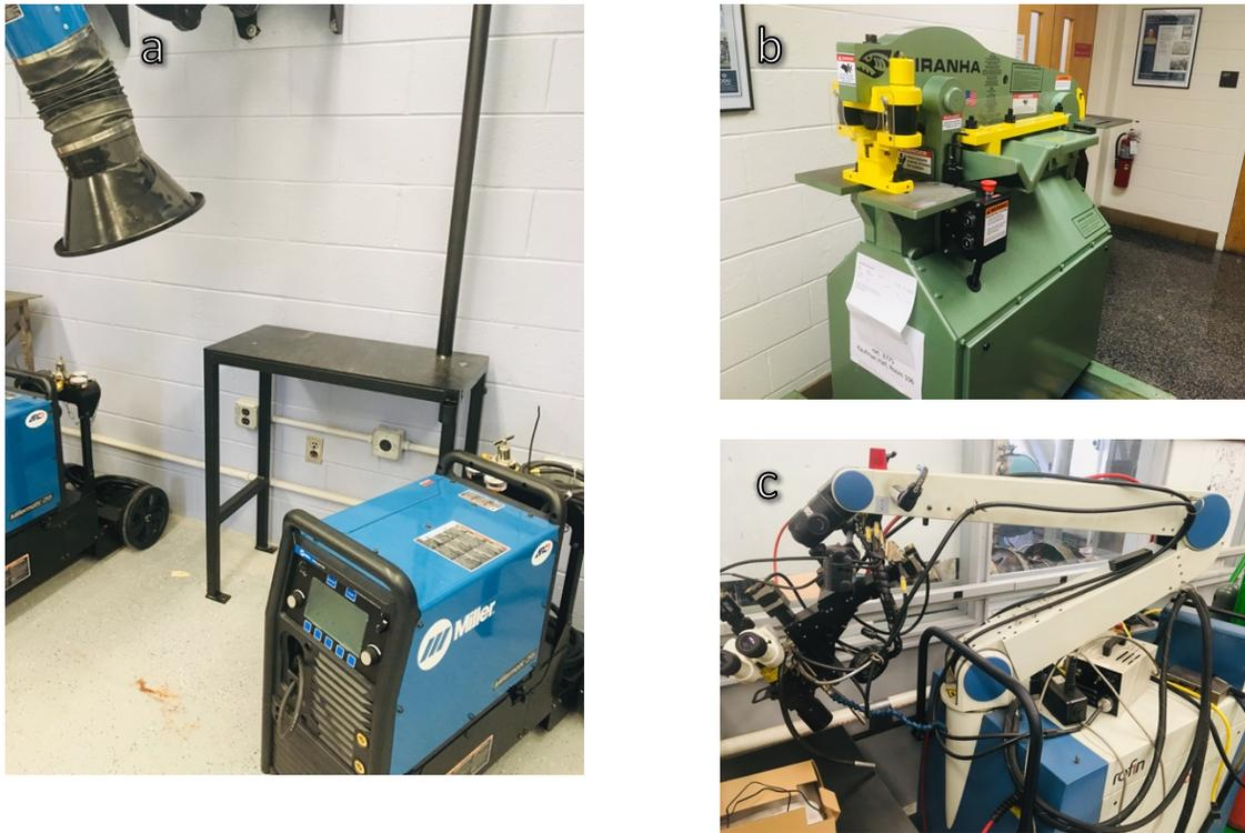
Figure 1. Some of the welding equipment used in LWP: a. ventilation system with GMAW machine; b. Piranha Ironworker machine; c. laser welding machine.
