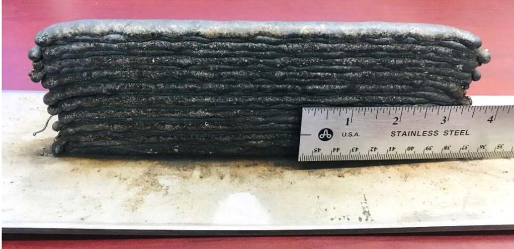
Figure 3. WAAM samples built from 304 stainless steel
