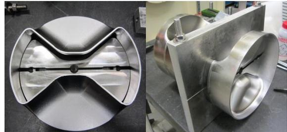
Figure 6: Weld fixturing.
