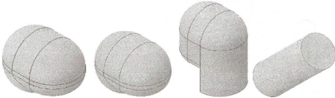
Figure 3: Second Solid Modeling Attempt using Autodesk Inventor (from left to right: brain, CSF, skull, and impactor)
