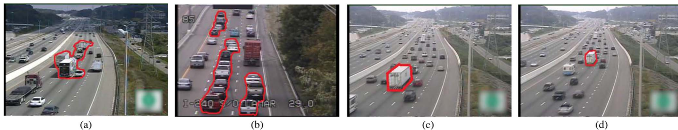
Fig. 1. Examples of image frames. (a) and (b) show the severe occlusions. (c) and (d) are two consecutive image frames showing strong shape distortion caused by the foreshortening effect. Feature points or edges are often unreliable in these low resolution images.
