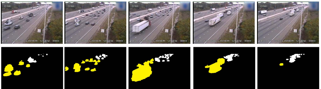
Fig. 9. Five consecutive image frames and their corresponding foreground segments. Yellow segments contain unclassified vehicles and white segments contain classified vehicles that have been classified in previous frame. All the segments are extracted from the pre-defined region of interest.
