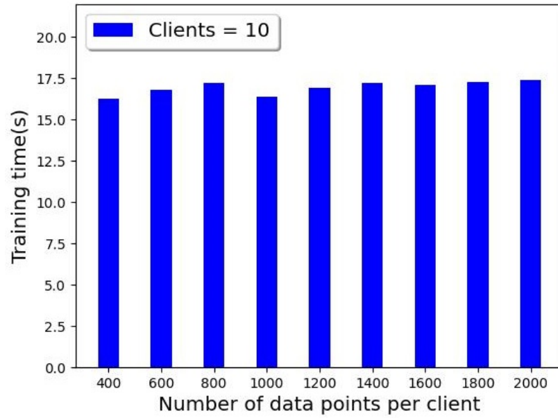
Figure 25. Total training time of aggregator after 25 rounds when |C| = 10 , for varying numbers of data points per client.
