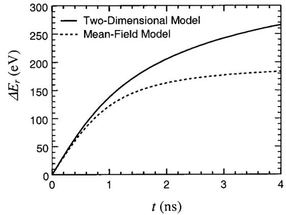
FIG. 4. The relative value  $\Delta E_r$  of electron energy spread as a function of the EP drift time  $t$  for initial EP duration of  $\tau=1000$  fs, electron initial energy of 30 keV,  $r_b=0.1$  mm, and  $N=5000$ , in the cases of the MF theory and the 2D model.
