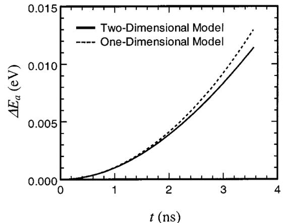
FIG. 5. The absolute value  $\Delta E_a$  of electron energy spread due to space-charge effects as a function of the EP drift time  $t$  for initial EP duration of  $\tau=100$  fs, electron initial energy of 30 keV,  $r_b=0.4$  mm, and  $N=3000$ , in the cases of 1D and 2D models.
