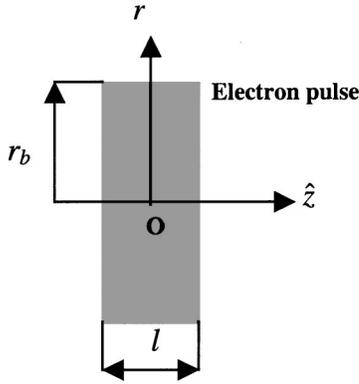
FIG. 1. An electron pulse disk simulating a drifting femtosecond photoelectron pulse.
