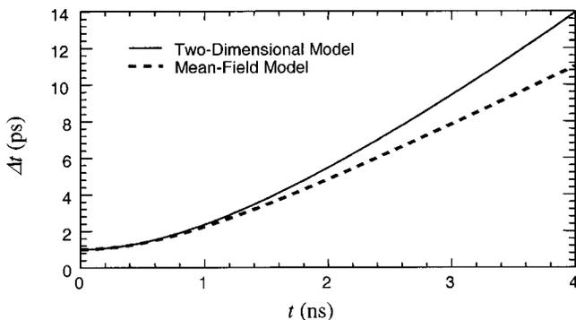
FIG. 3. The EP broadening  $\Delta t=l/v_b$  is plotted as a function of EP drift time  $t$  for initial EP duration of  $\tau=1000$  fs, electron initial energy of 30 keV,  $r_b=0.1$  mm, and  $N=5000$ , in the cases of the MF theory and the 2D model.
