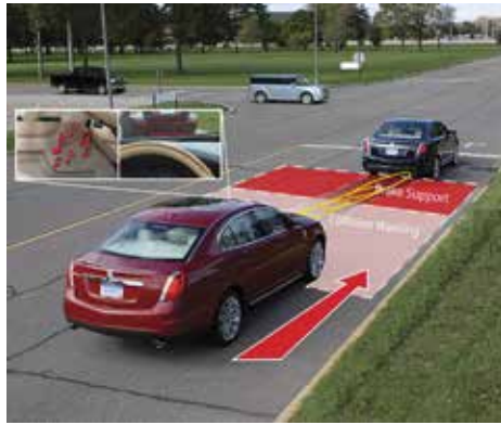
Photo 5. Advanced Driver Assistance System. The Controller Area Network (CAN) is an IoT automobile computing system. The illustration shows how the system can warn of a stopped car and automatically brake to avoid an accident. Credit: Wikimedia Commons.
