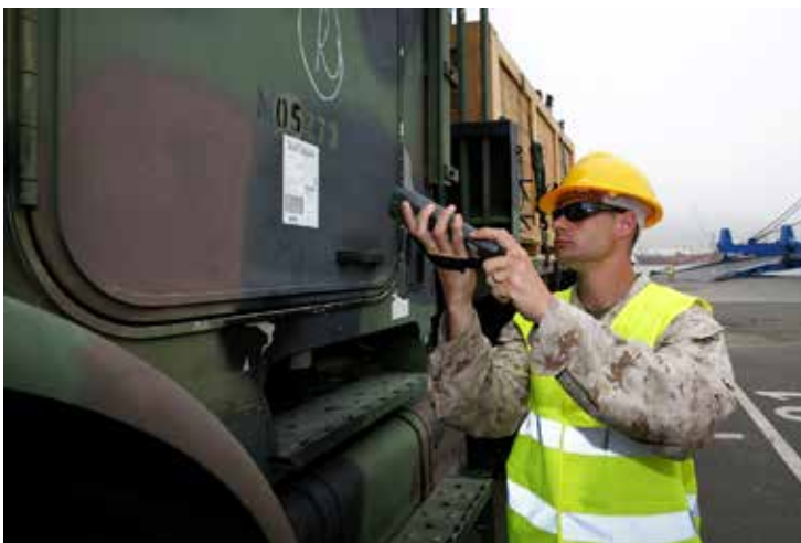
Photo 7. RFID Tagged Truck. Before the advent of IoT sensors, railroad and trucking companies attached RFID (radio-frequency identification) tags to trailers and railroad cars to track them. RFID has short range connectivity. IoT monitors can be tracked using the internet from much greater distances. Credit: U.S. Marine Corps.
