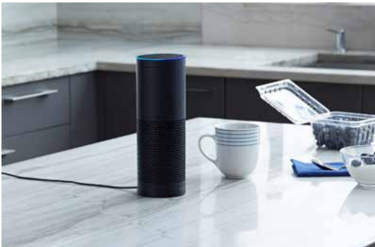
Photo 2. Amazon Echo. The Amazon Echo and Dot are Internet of Things devices. Google Home is a similar product. These products can control home products such as lightbulbs and fans. They can also provide information by asking their assistants questions such as the latest sports scores. Credit: Amazon.
