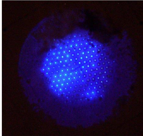
Fig. 3. Emission of 425 nm photons using UV excitation on opposite end of fiber; liquid loss from the fiber end results in no emission.
