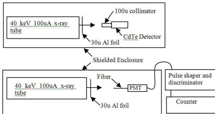
Fig. 4. Placement of CdTe detector and collimator for characterization of x-ray tube and taking fiber data.
