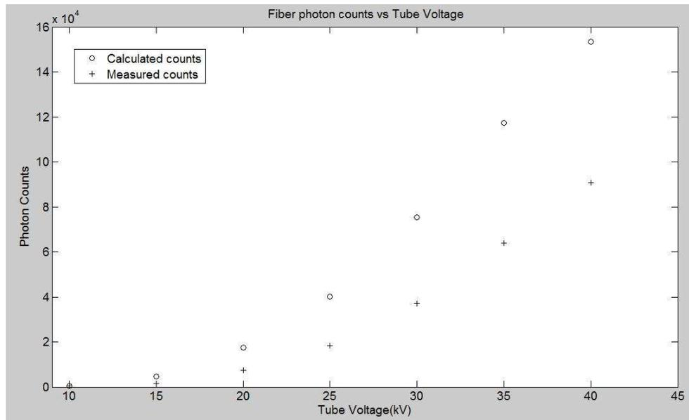
Fig. 5. Fiber photon counts versus tube voltage comparing calculated with measured counts.
