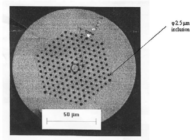
Fig. 1. Microstructured quartz optical fiber cross-section. Total fiber diameter is 125 microns with 168 air filled inclusions. These inclusions become fiber cores when filled with scintillator material.
