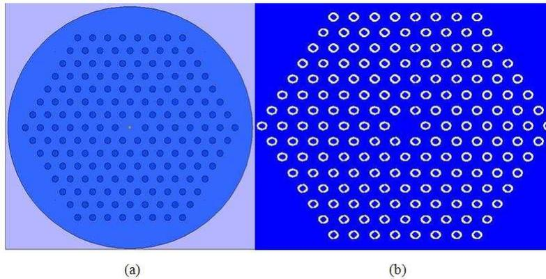
Fig. 2. (a) FIMMWAVE FEM model geometry, (b) CUDOS multipole model geometry. Note the center hole in the FIMMWAVE model is filled by using cladding material.
