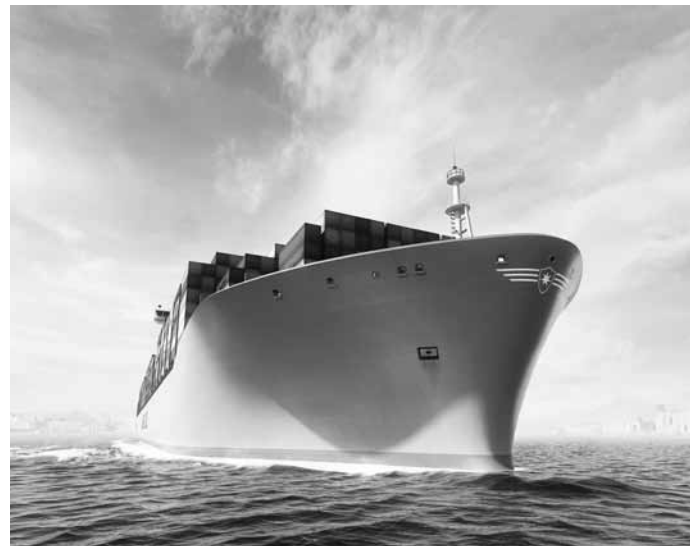
Figure 1. The Maersk’s Triple E is the world’s largest container vessel. It represents a milestone in improvements in fuel efficiency and environmental friendliness. The ship achieves its efficiencies through innovative design features such as a smaller twin-engine and twin screw design. While the Triple E cruises the oceans at slightly slower speed than its counterparts, it does so with a nearly twenty percent increase in fuel economy. (Photo Credit: Maersk)
