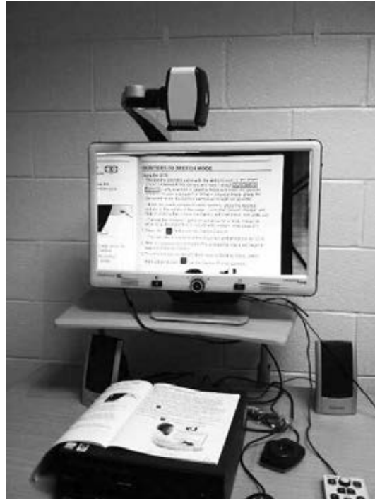
Photo 2. The da Vinci vision system integrates a Sony® HD camera with software applications that enable an individual to magnify and view printed materials in color and varying contrasts with a high degree of clarity. Also, the system has optical character recognition and text-to-speech capabilities.
