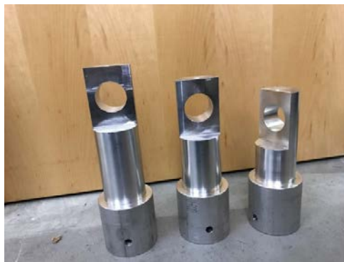
Figure 7. Three Common Couplers (10", 9", and 8" long)
