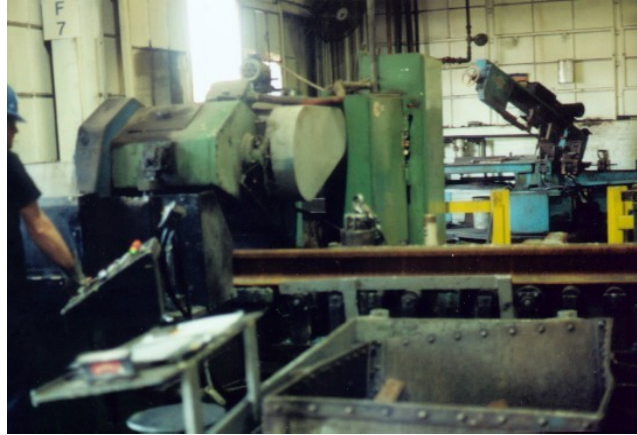
Figure 4. A Rail Being Cut into Required Lengths for Use in Frog Manufacturing
