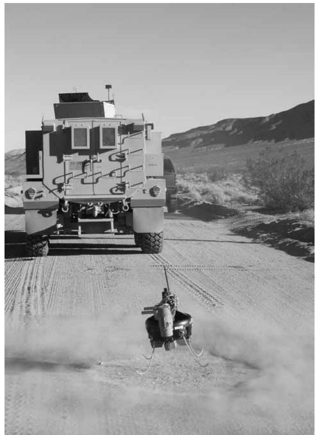
Figure 2. As military planners, scientists, and engineers as well as terrorists develop new weapons, researchers are looking for ways to counter those weapons with new technologies. Shown here is a Foster-Miller Talon Mk.II searching an area while a Micro Air Vehicle (MAV) provides a 360-degree view as the two work together to search for a simulated improvised explosive device (Credit: Naval Air Warfare Center Weapons Division). [See www.navair.navy.mil/naw-cwd/nawcwg/media_galleries/photos/photos_technology.htm ]
