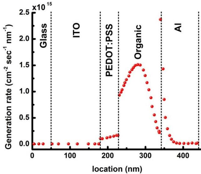
**Figure 1.** Generation of excitons simulated using TMM model.
