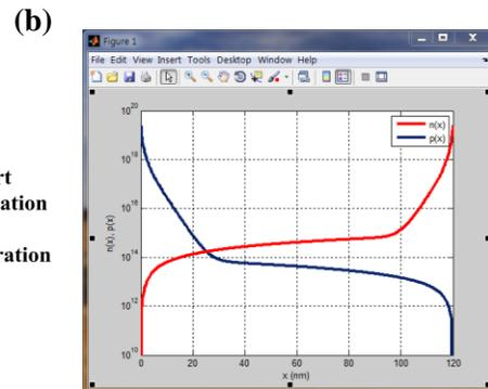
**Figure 2.** (a) Photoconversion process and (b) distribution of charge carriers inside an organic solar cell.
