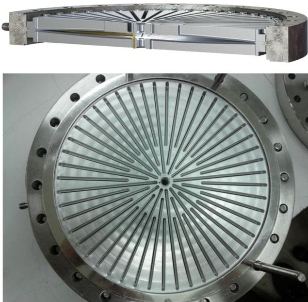
FIG. 1. Top: cut-away view of the harmonically resonant cavity. Bottom: photograph of the cavity nested inside the bore of a 10" double-sided knife edge Conflat flange. Two additional 10" Conflat flanges attach to either side to form the UHV-compatible vacuum vessel.
