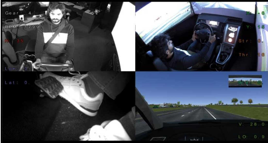
Figure 2. Four synchronized views on SimObserver
