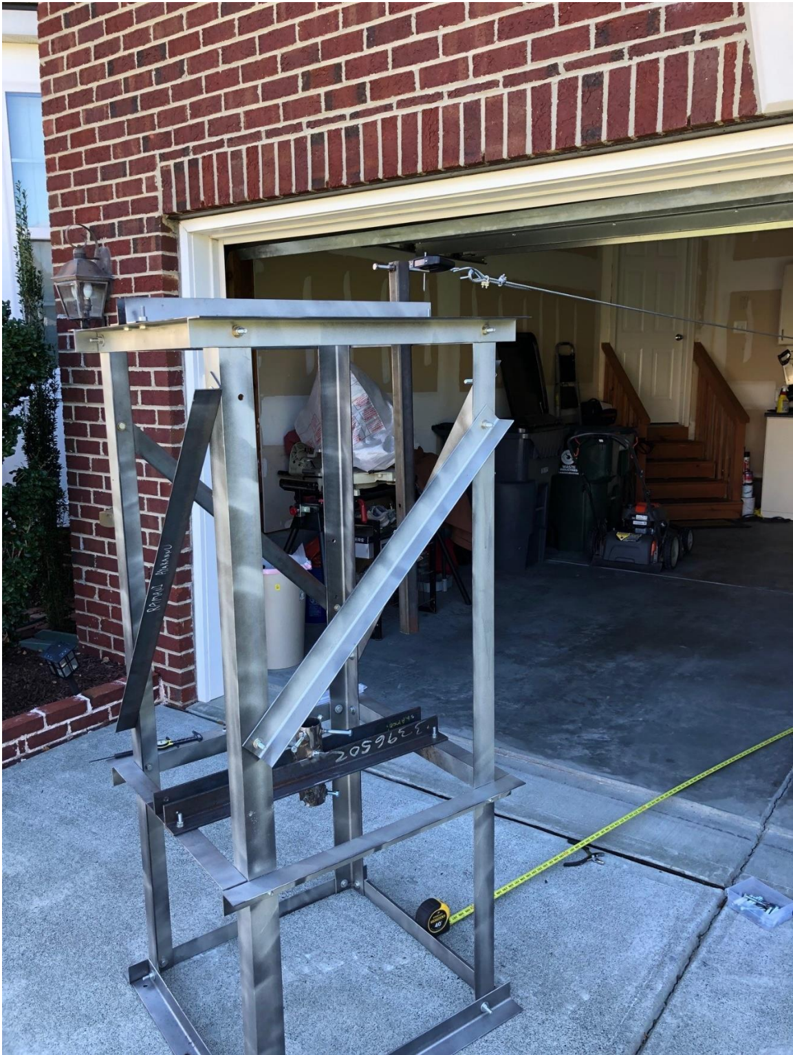
Figure 6-4. Test Frame with Cable and Digital Load Gage
