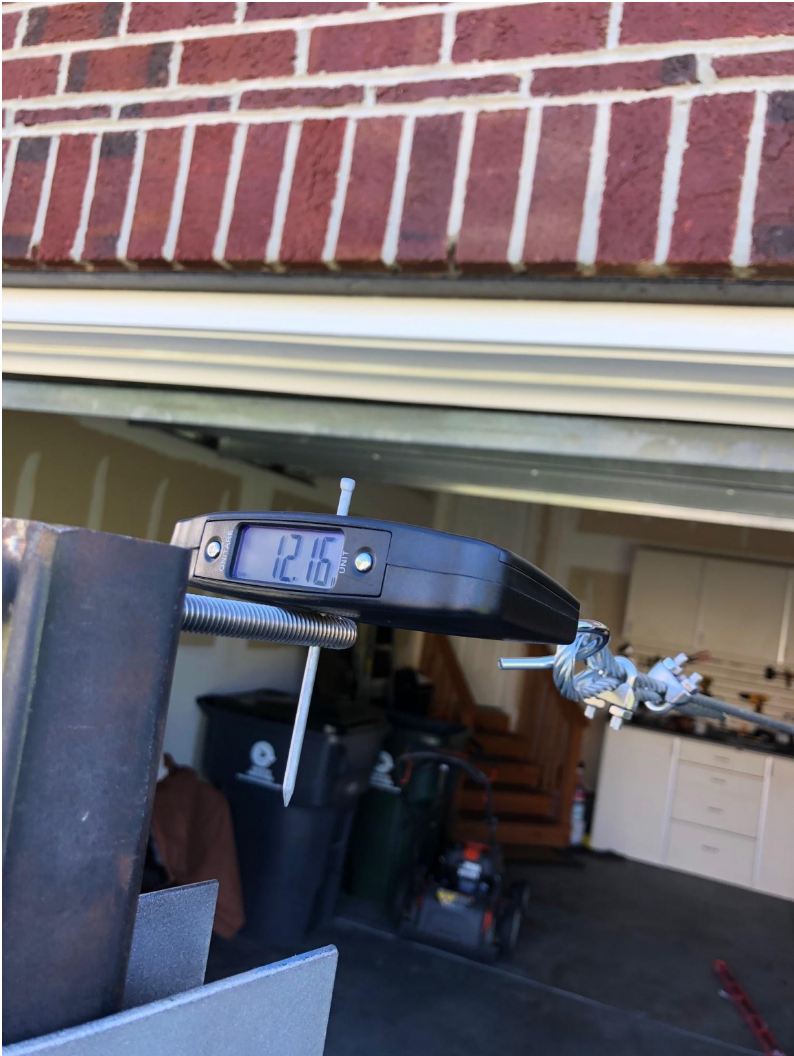
Figure 6-6: Digital Load Gauge to Measure Cable Tension
