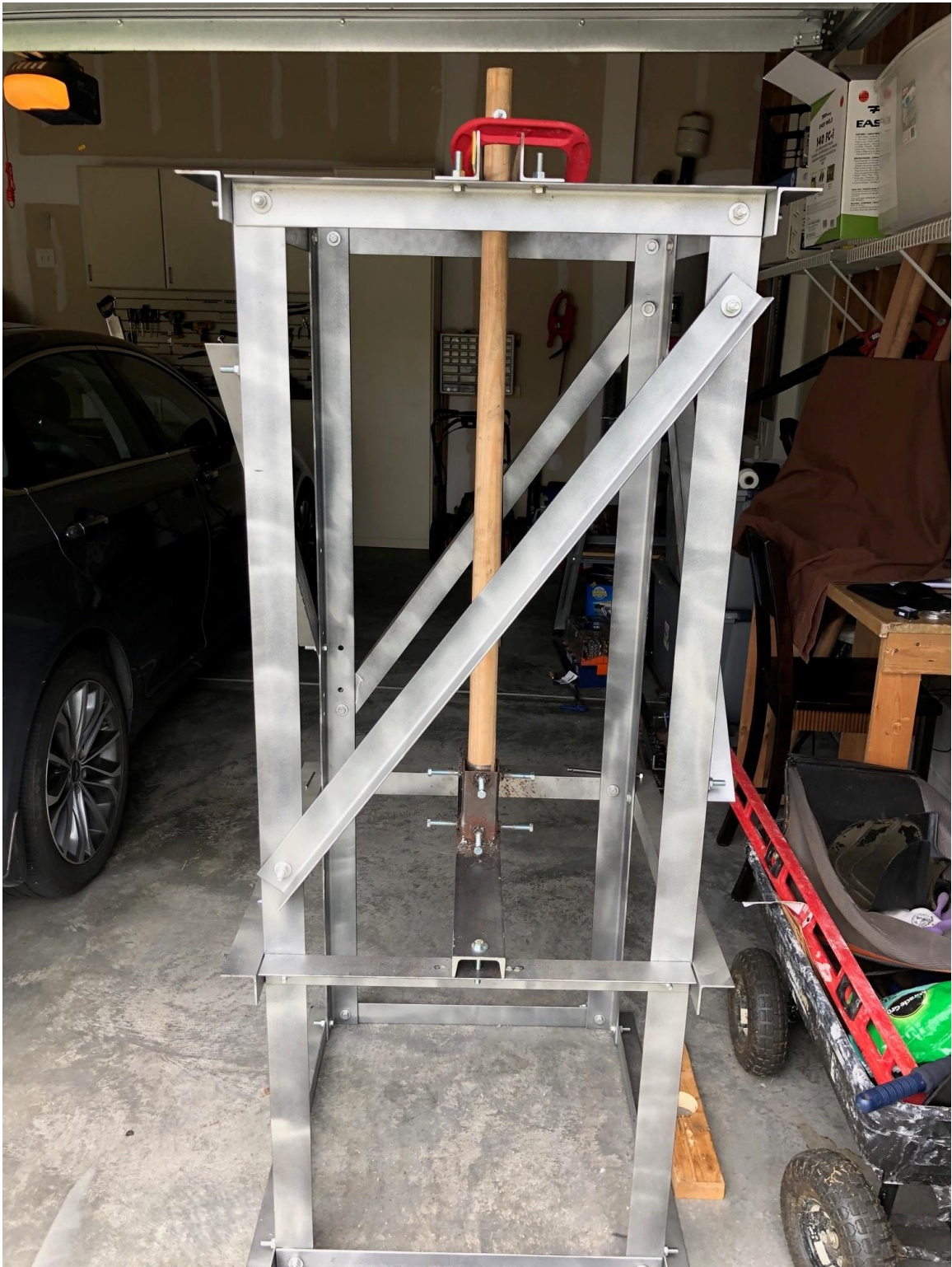
Figure 6-5: 4' 0" Test Specimen and Base Connection
