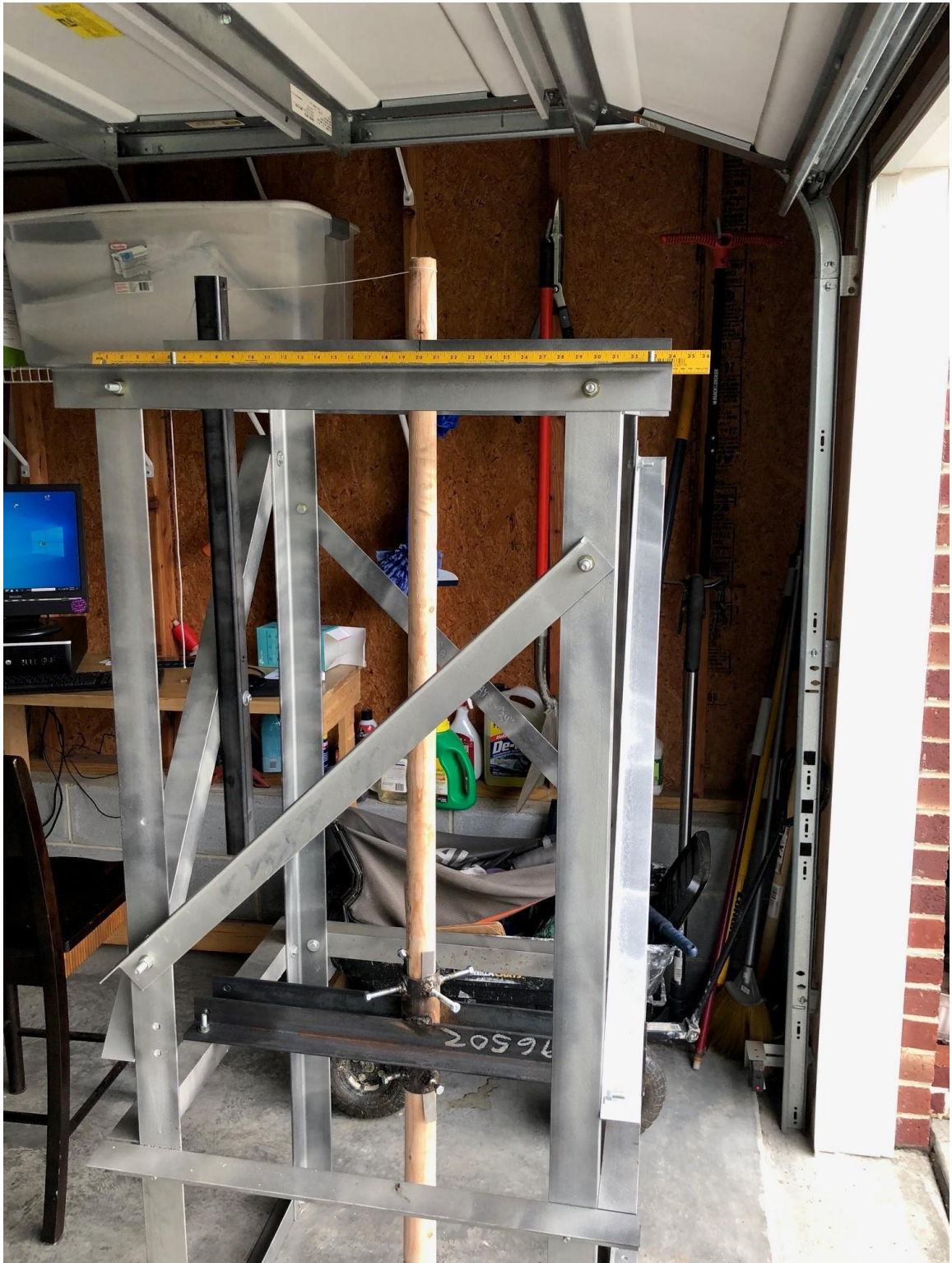
Figure 6-7. 6' 0" Test Pole with Fixed Base Attachment
