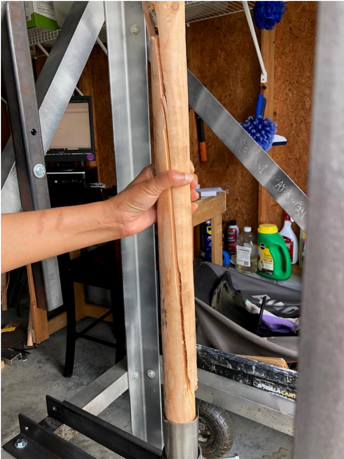
Figure 6-9: Test Pole Failure Profile
