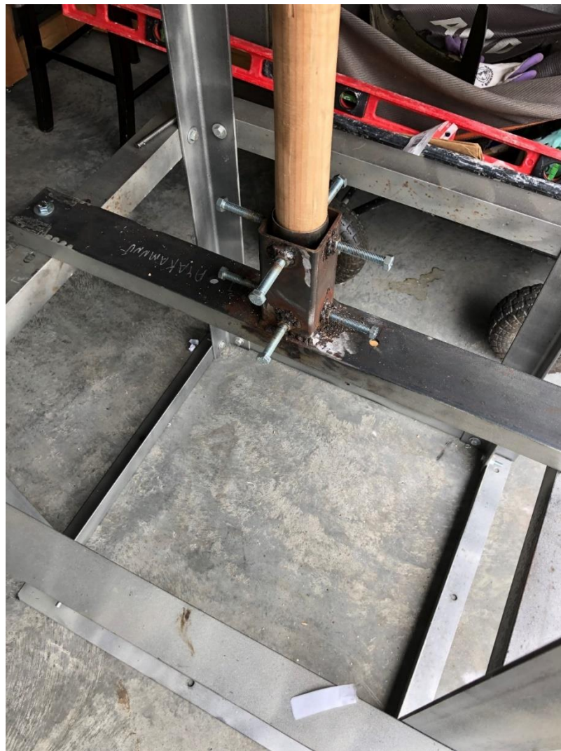
Figure 2-7. Fixed Base Condition -Option 1 Base Connection
