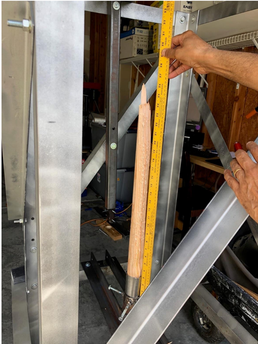
Figure 6-10. Test Pole Breakage Measurements
