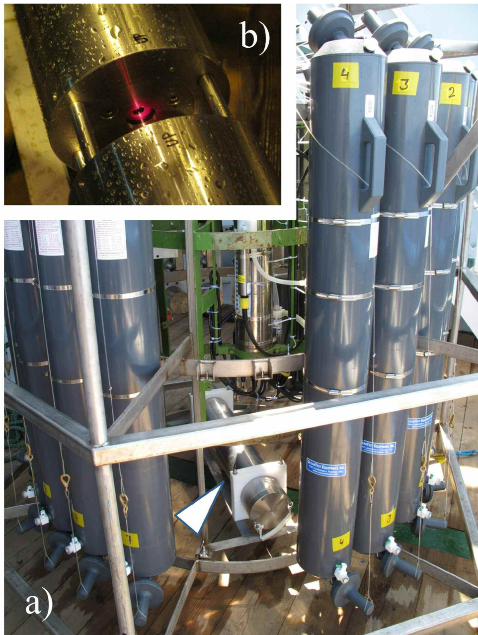
Fig. 2. Mounting of the DIHM on the CTD frame (a) and close up of the camera port reflecting the red laser light (b). The overall length of the DIHM is 137 cm.
