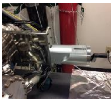
Fig. F.17 Change pressure to 3 \times 10^{-3} torr by changing gate valve position
