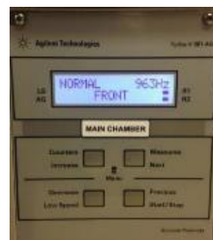
Fig. F.8 Frequency of the turbo pump should reach 963 Hz
