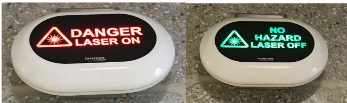
Fig. G.6 Illuminated indicator outside the room.
