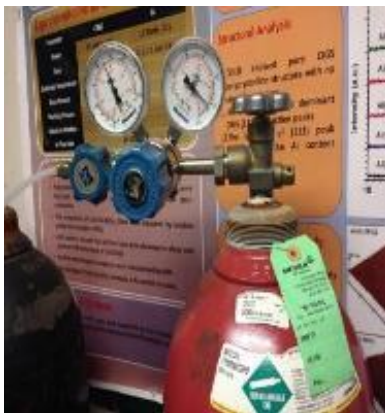
Fig. F.10 Ar gas valve on
