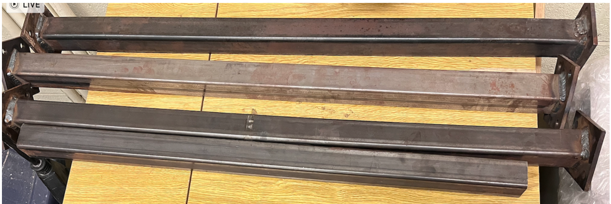
Figure 17. A513 Type -1 Beam-Column Specimens
