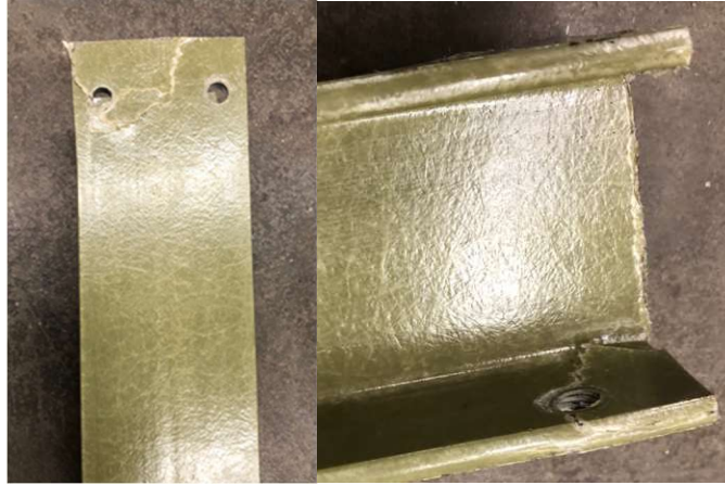
Figure 68. Cracks Due to Stress Concentration
