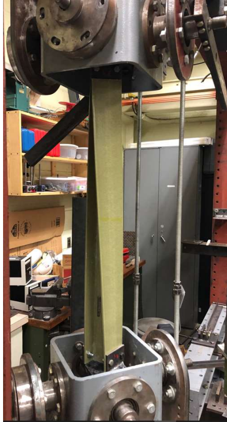
Figure 44. Specimen under Torsional Moment for Test T-1
