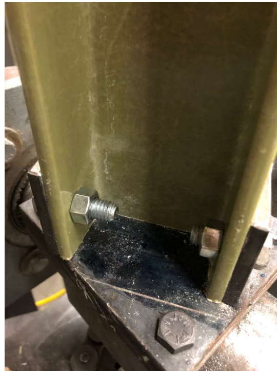
Figure 43. Bottom End Connection of the Specimen
