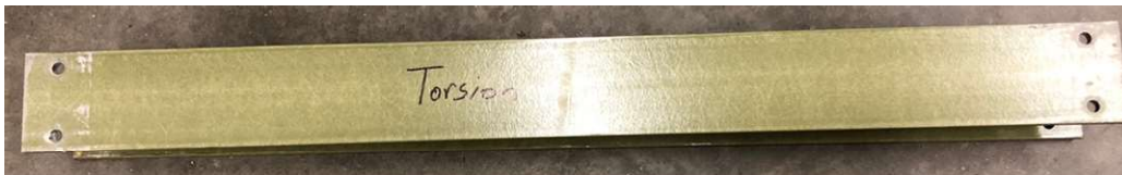
Figure 47. Specimen Shape One Week after Torsion Test T-1
