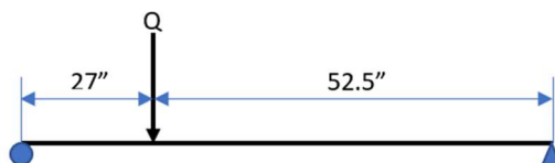
Figure 100. Applied Load, Q at 27 in. from the Support
