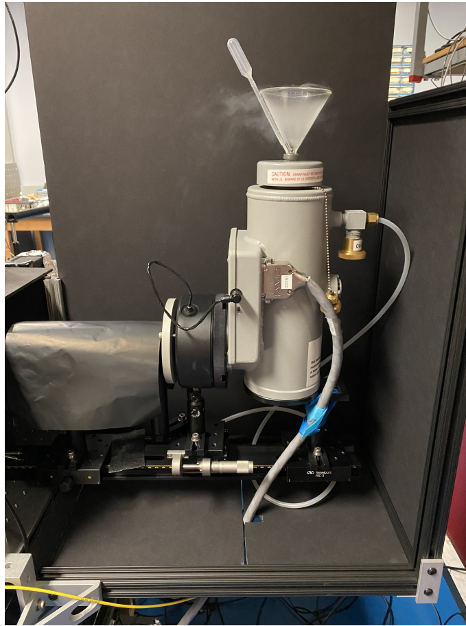
FIG. 17: Photograph of the LN CCD during liquid nitrogen filling.
