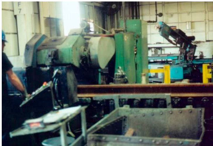
Fig. 4. A Rail being cut into required lengths for use in frog manufacturing
