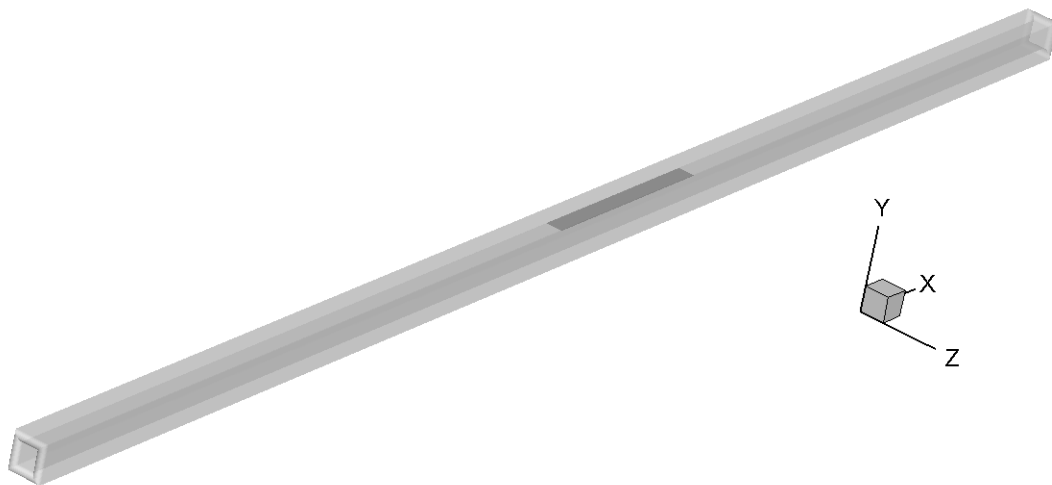
Figure 2. Modeling of an internal ducted environment as an external scattering problem. Liner section inside the duct is noted by the darkened area.
