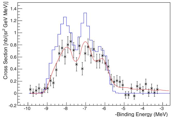
FIG. 3. (Color online) The <sup>9</sup>Li differential cross section as a function of the binding energy. Experimental points vs Monte Carlo results (red curve) and vs Monte Carlo results with radiative effects turned off (blue histogram).
