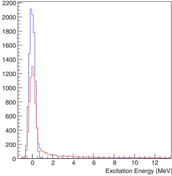
FIG. 5. (Color online) One peak of the excitation energy spectrum of the hypernucleus  ${}^9_\Lambda\text{Li}$  obtained through the reaction  ${}^9\text{Be}(e, e'K^+){}^9_\Lambda\text{Li}$  as predicted by the Monte Carlo SIMC when including all effects (red curve) and “turning off” the radiative effects (blue curve). Arbitrary units. The position of the peak has been made coincident with the ground state.
