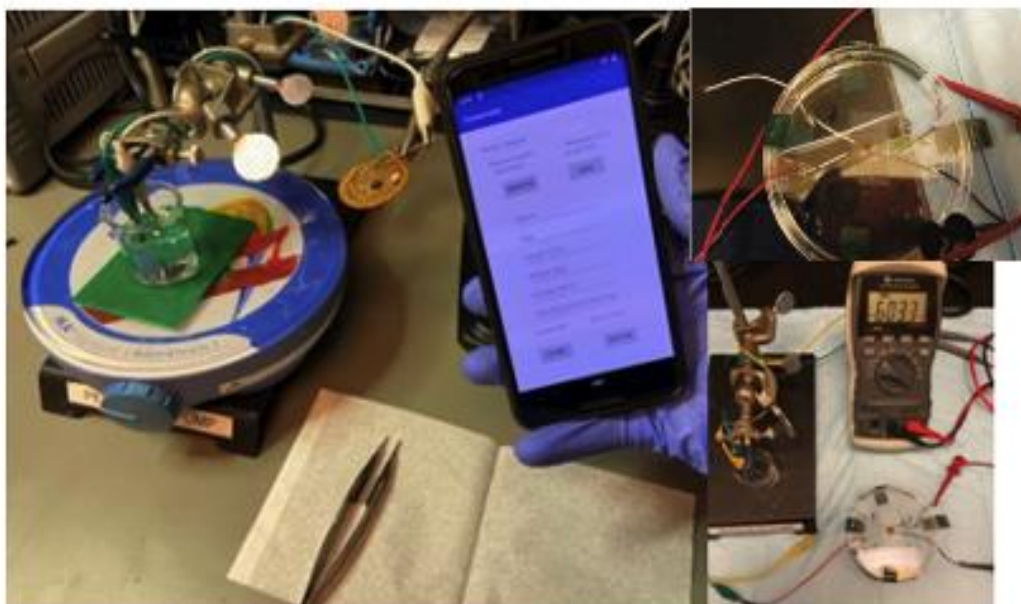
Figure 54. Assembled fuel cell setup with NFC/smartphone data recording and with voltage measurement using multimeter.
