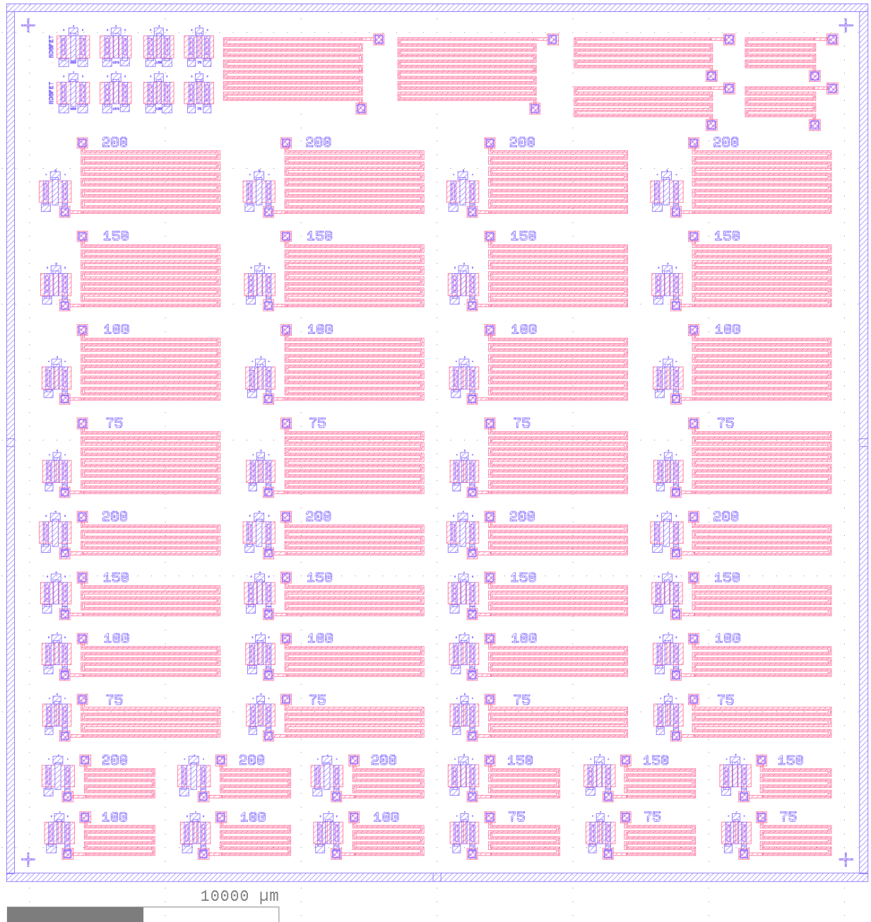
Figure 32: KLayout design featuring various transistor channel lengths (200 \mu\text{m} , 150 \mu\text{m} , 100 \mu\text{m} , and 75 \mu\text{m} ) and resistor combinations.
