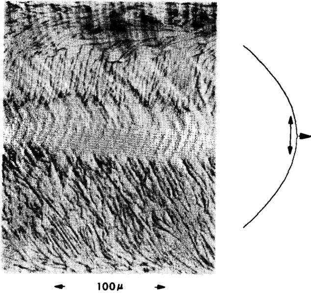
FIG. 5. Optical micrograph of a continuous Si film on SiO<sub>2</sub> recrystallized by a laser beam oscillating at 1400 Hz in the direction of the slow table motion and at 700 Hz in the other axis. The trace of the oscillation is shown at right.
