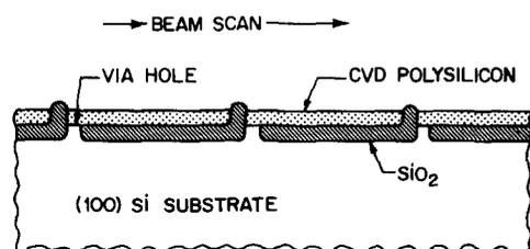
FIG. 1. Schematic cross section of Si islands recessed into SiO<sub>2</sub> "crucibles," with via links to the substrate.
