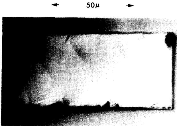
FIG. 3. Optical micrograph of a single crystalline via island produced by rapidly oscillating laser beam.
