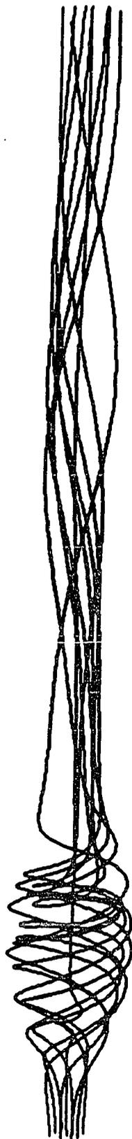
Fig. 5.7 Vortex lines for flow with vortex breakdown.
