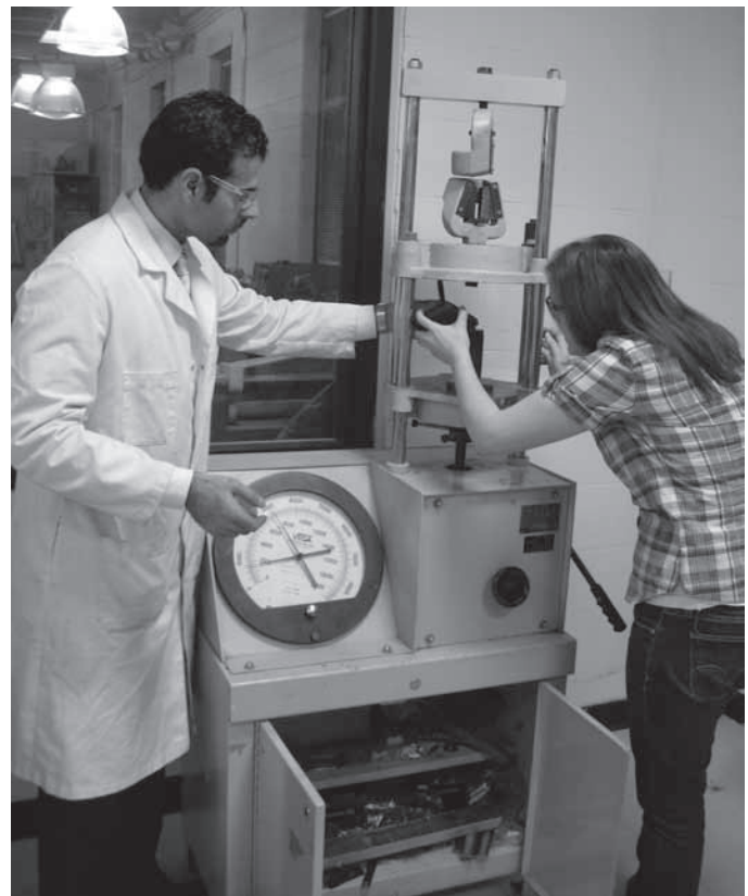
Figure 3. Here the student is getting the equipment ready for a compression test of a material. Brittle materials will fail suddenly after their ultimate strength is exceeded. These brittle materials have much greater compression strength than tensile strength. That is why these materials are mostly tested in compression. Credit: Author.
