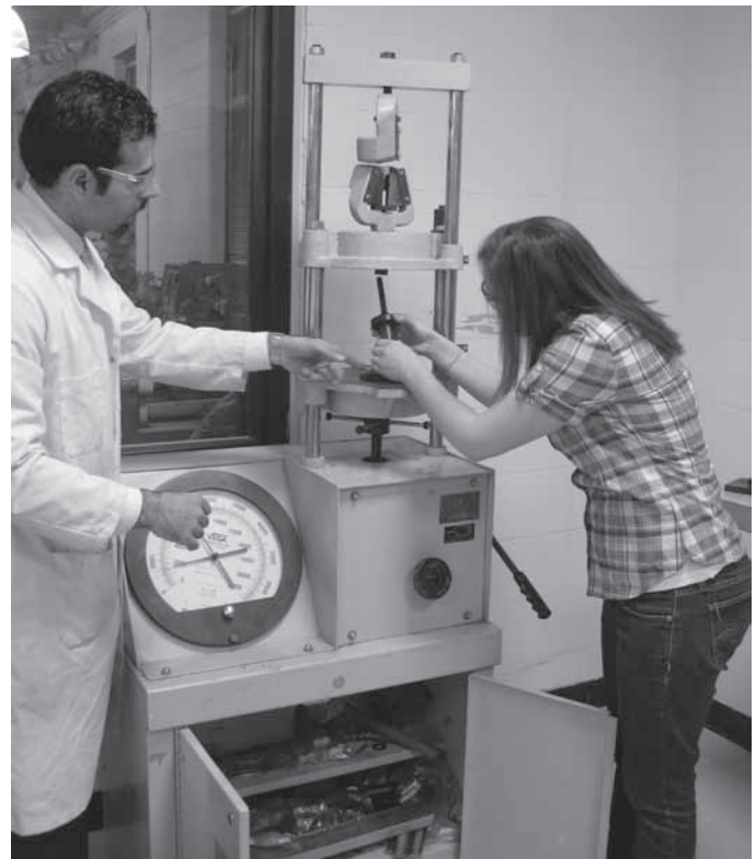
Figure 4. Getting the equipment ready for shear testing. Shear testing results are not as precise as tension and compression testing because of the additional introduction of friction and bending forces in the testing process. Fasteners such as bolts, rivets, and screws are typically associated with shear stresses. Credit: Author.
