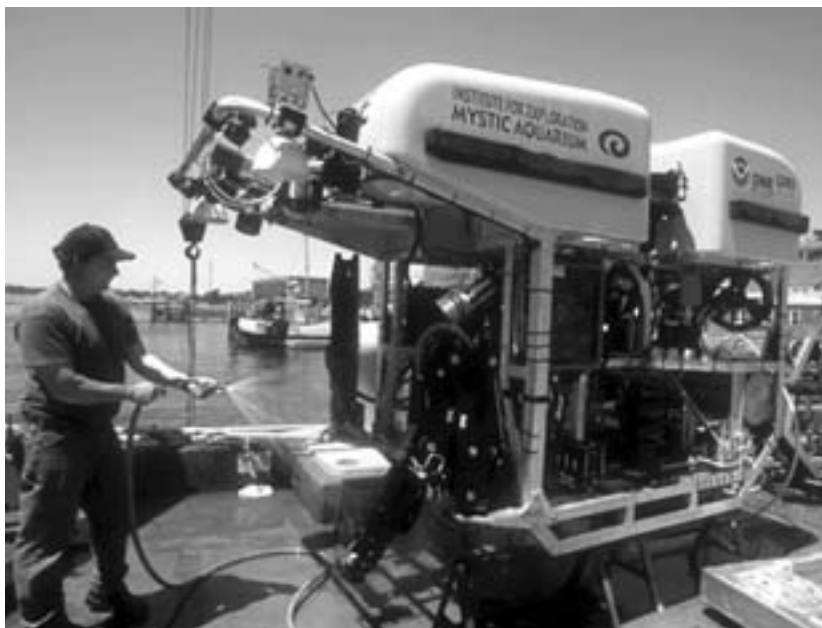
The Hercules ROV was specially designed to conduct underwater archaeological surveys at dive sites in the Black Sea. Photo courtesy of J. Weirich.
