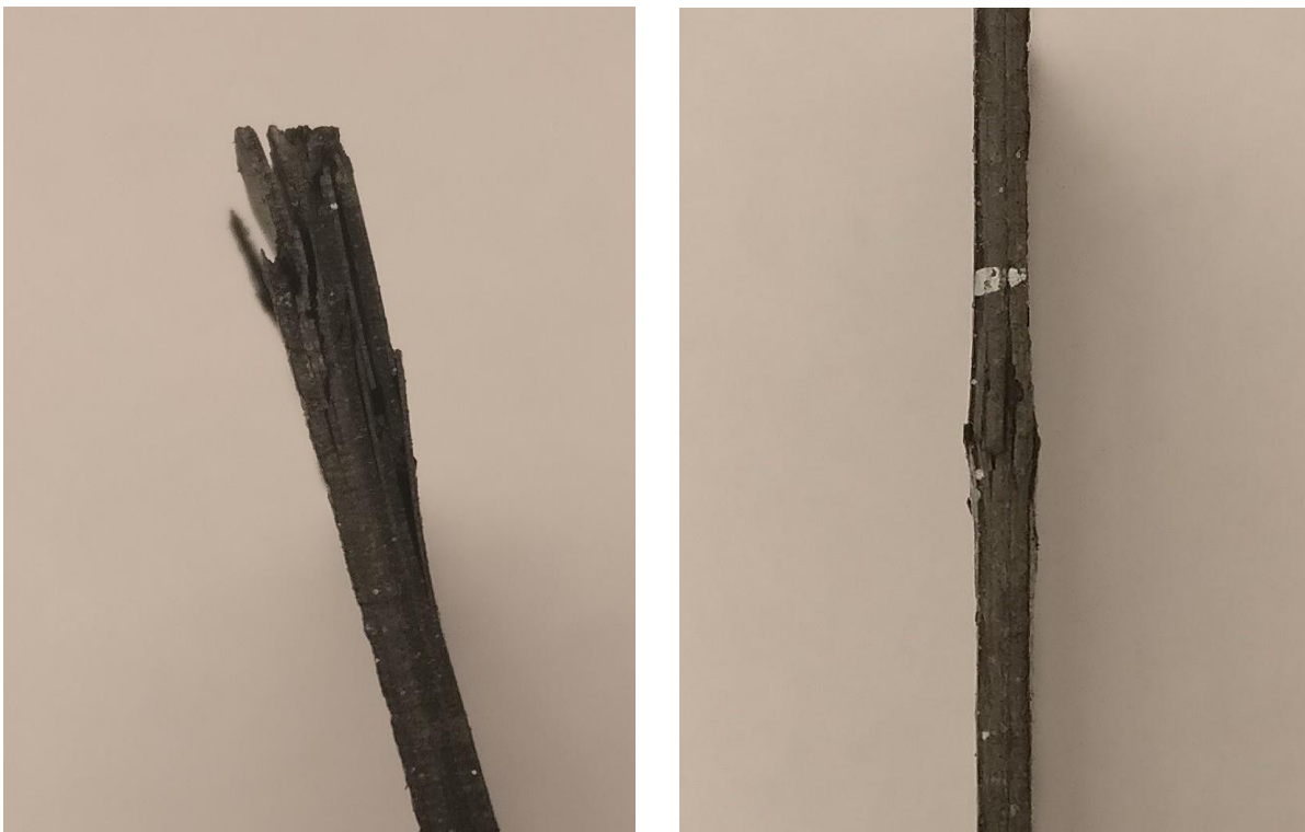
(a) Brooming of the loading edge of a specimen. (b) Pinching of a specimen edge.
