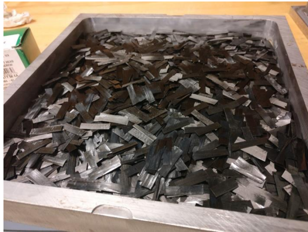
Fig. 6: Mold used to make 254 mm plate filled with platelets.
