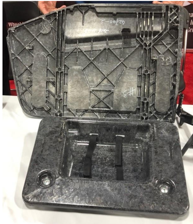
Fig. 2: Airplane seat made of prepreg platelet molded composites at ACCE 2019.
