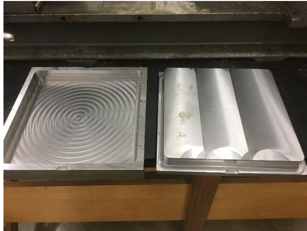
Fig. 5: Mold used to make 254 mm plate.
