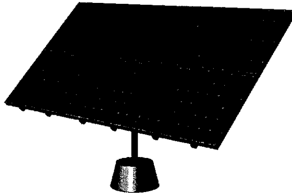
Figure 2.4 Dual-Axis Photovoltaic Tracker
