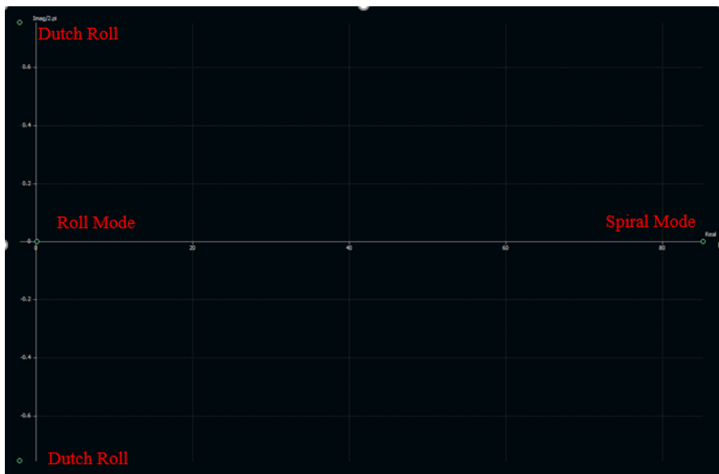
Figure 73-Root locus plot for lateral modes for EdgeTRA
