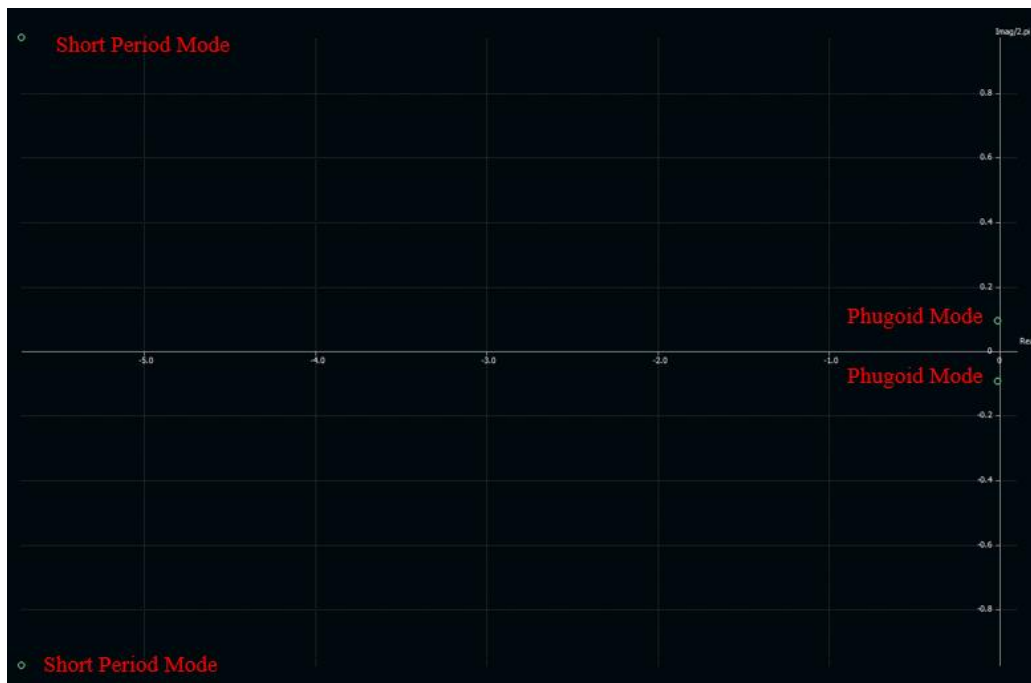
Figure 72-Root locus plot of longitudinal modes for EdgeTRA
