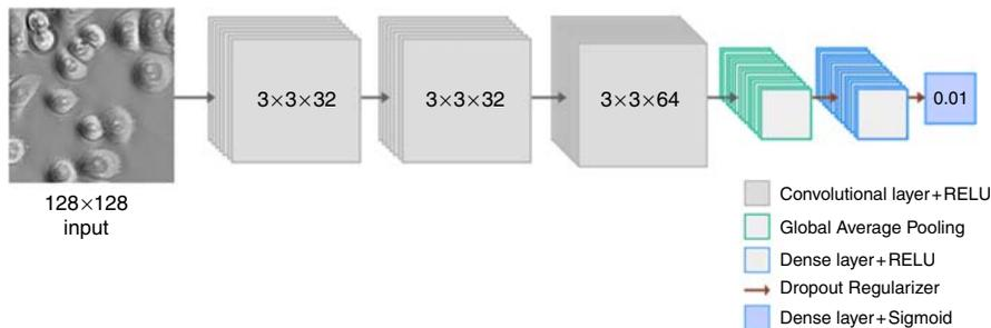
**Notes:** The model propagates the input image through its four hidden layers and then outputs predicted probabilities between 0 and 1, represent both MDA-MB-468 and MCF7 classes respectively, with the threshold being 0.5. This example accurately outputs 0.01, which represents MDA-MB-468 cell class
